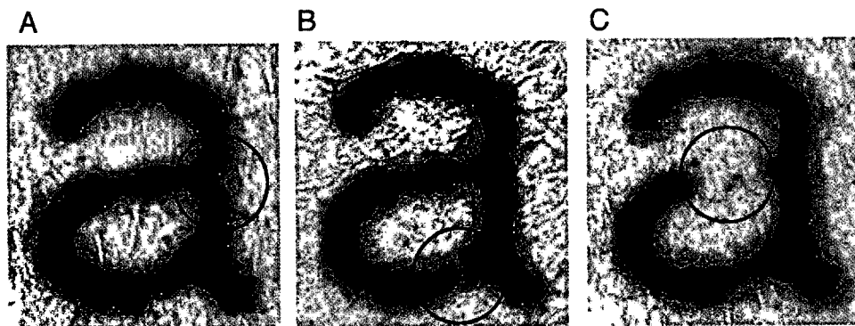
Figure 1. Examples of three categories of toner flaking where defined A = chipped; B = cracked; and C = section missing.
