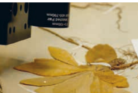
Figure 4. Specimen during microfading test. The diameter of the spot is 0.6mm.
