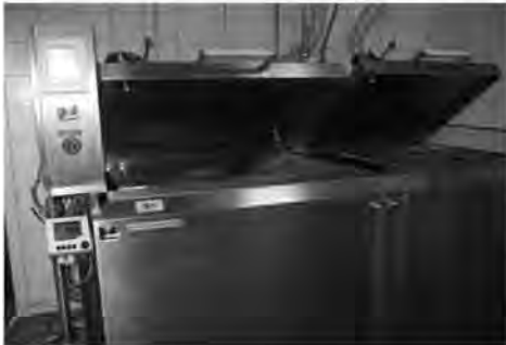
BMU 1360-2 Bone Maceration Unit w. 2 Process Chambers
