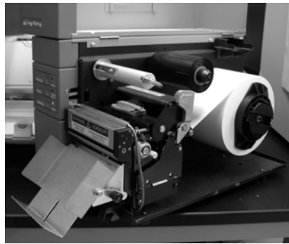
Figure 2: Datamax Prodigy Max 300 printer opened, showing internal components and loaded media and ribbon.
