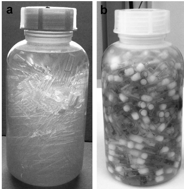
Figure 2. Comparison of experimental sample with actual sample from a natural history collection. (a) soda lime glass sample from comparative sample pair (CSP) D; (b) 2-L polyethylene bottle with glass vials containing Diptera specimens from the wet collection of the Zoologische Staatssammlung in München.
