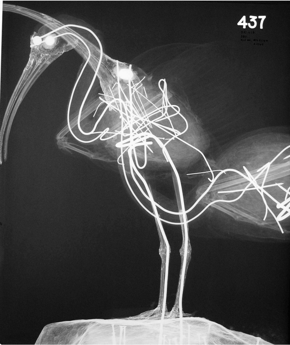
Figure 8. X-radiograph from a pair of Scarlet Ibis ( Eudocimus ruber ) NH.Z.289 and 290 showing metal armature.
