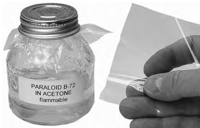
Figure 4. A baby formula jar. The lid is screwed down over a small square of silicone-coated Mylar to prevent sticking.
