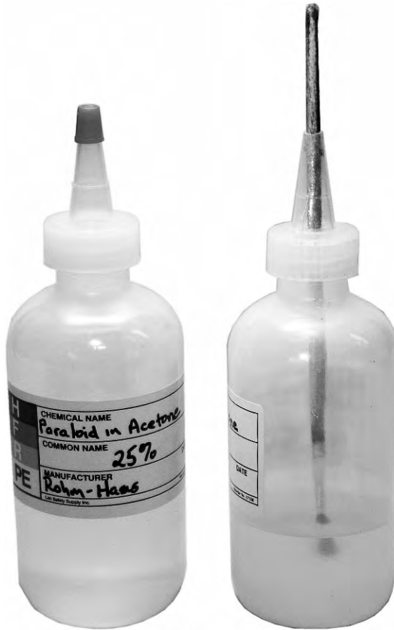
Figure 10. A low-density polyethylene bottle with a Yorker cap. The bottle on the right is outfitted with a solvent-proof brush.
