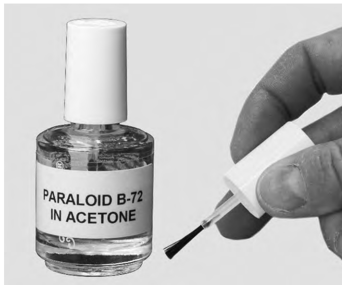
Figure 9. For dispensing thin solutions, clear nail-polish bottles are very convenient (rinsed well, refilled, and relabeled).
