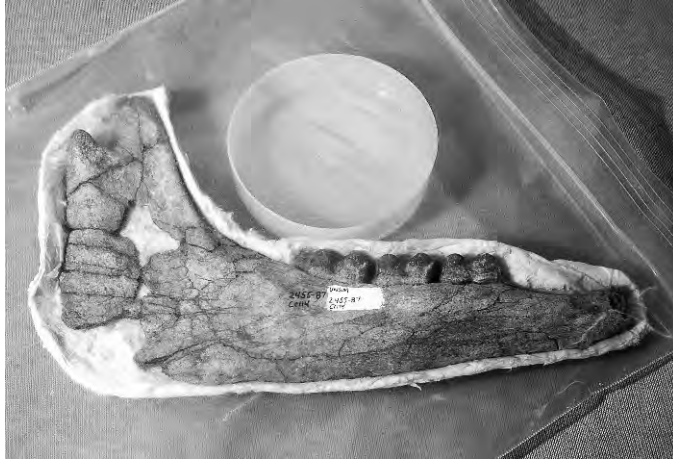
Figure 13. A simple vapor chamber made from a polyethylene bag filled with fumes from open dishes of solvent.
