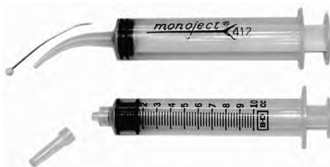
Figure 7. Syringes for thick and thin solutions: (top) Monoject™ 412, stopped with a ball-headed sewing pin; (bottom) a BD Luer-Lok™ syringe with Luer-Lok™ tip.
