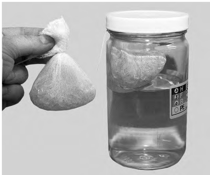
Figure 5. An easy way to mix Paraloid B-72 by suspension in a cheesecloth bundle tied with sewing thread inside a glass jar partially filled with solvent.
