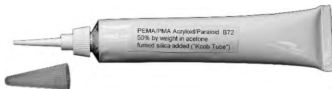
Figure 6. The “Koob Tube,” a self-loaded tube for dispensing thick solutions of Paraloid B-72 in acetone.
