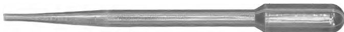
Figure 12. Disposable plastic droppers are equally useful in the lab and the field for dripping applications over large areas and into cracks and for squirting up into undercuts.
