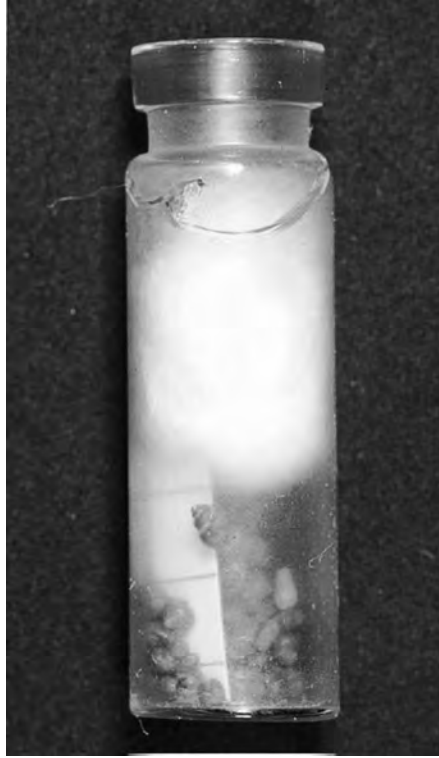
Figure 3. An old soda-glass vial showing the characteristic opacity and fracturing associated with glass disease.
