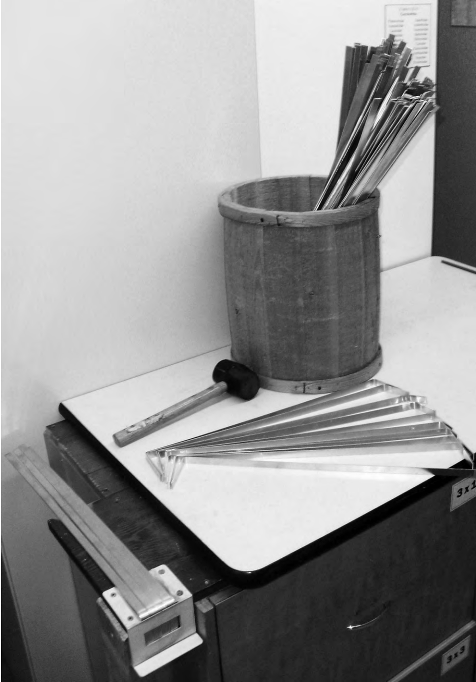
Figure 10. The bending jig (left) with raw and finished dividers.
