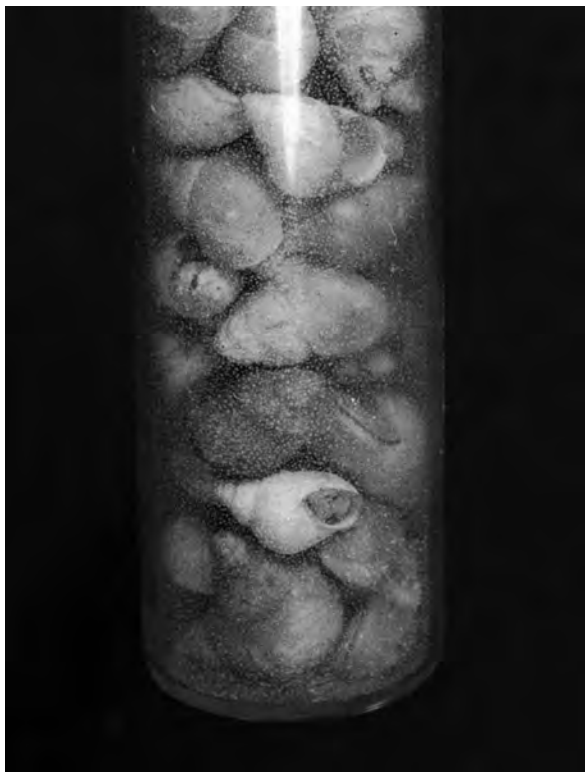
Figure 4. An old soda-glass vial, showing the formation of liquid droplets on the inner surface.
