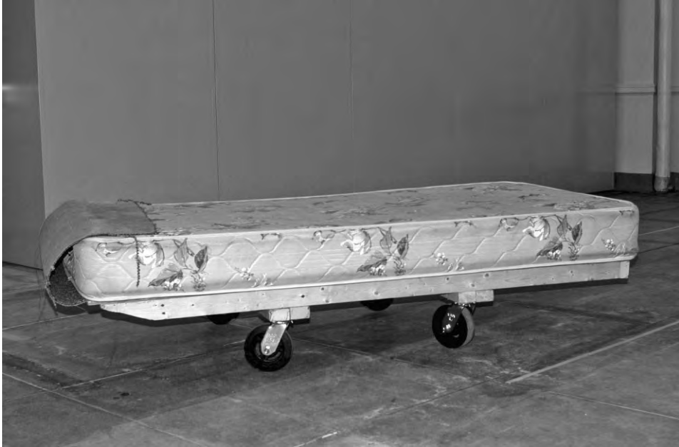
Figure 12. The “Dolly Parton” moving dolly. The strip of carpet at the sharp end was intended to be trapped by the cabinet and thus help hold the end steady, but proved unnecessary.
