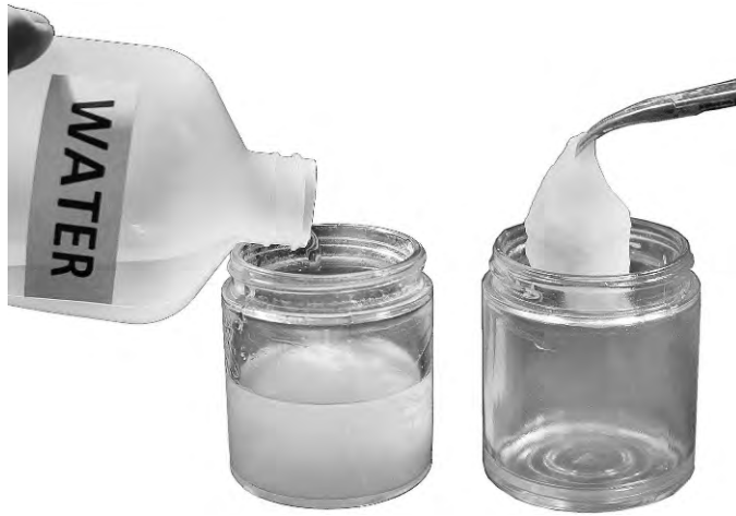
Figure 3. An easy way to clean glass jars by soaking in water before the solution has evaporated and peeling out the residue.
