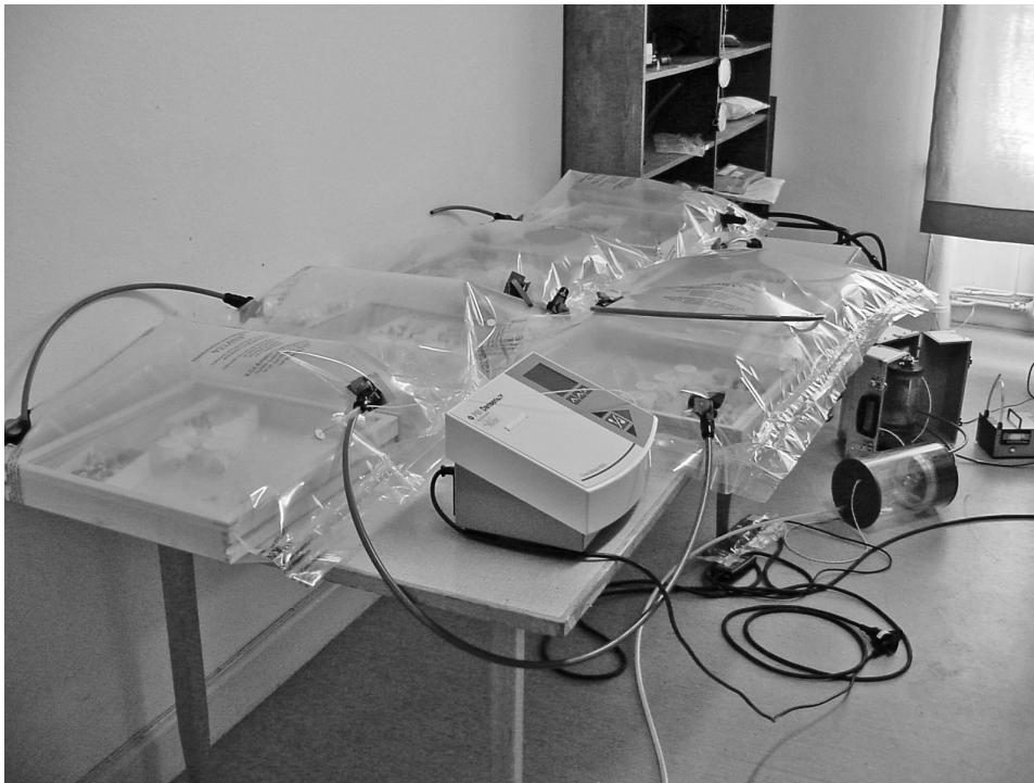
Figure 2. Anoxic treatment setup showing enclosures sealed in plastic that contain insect drawers and the valves through which nitrogen gas enters and exits. The Dansensor oxygen analyser is seen in the foreground.
