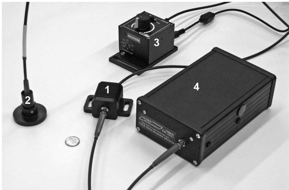
Figure 6. Prototype mini- microfade tester, GCI. (1) LED illuminator; (2) bifurcated lensless probe; (3) variable LED power supply; (4) spectrometer.
