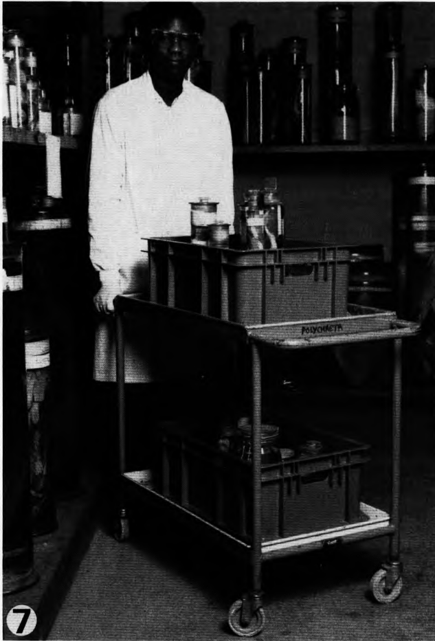
Figure 7. Tray trolley with plastic crates for stabilising jars during transportation of specimens.
